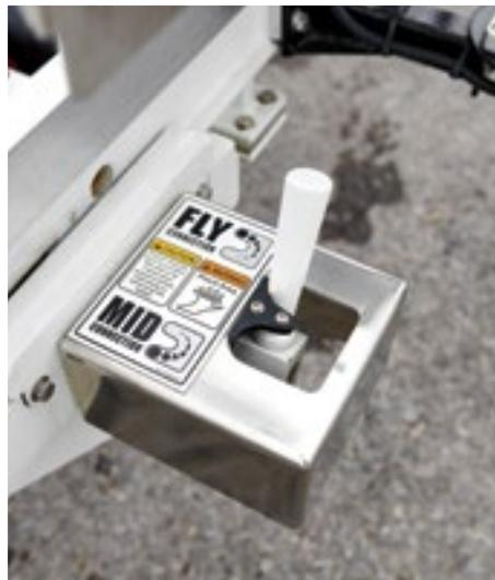
**WATERWAY CONTROLS:** Repositioning the waterway can be done easily with the flip of a mechanical lever.
