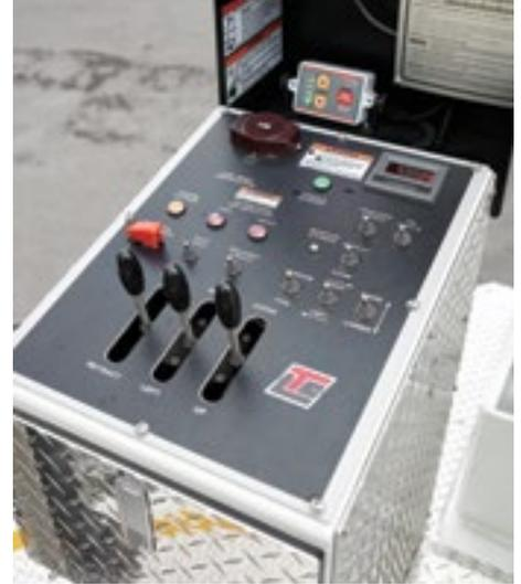
**SIMPLE CONTROLS:** Direct hydraulic control valves and hard-wired electric switches provide simple troubleshooting and worry-free operation.
