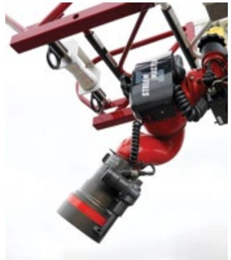
**WATER MONITOR:** When positioned at the tip, the water monitor can be elevated 30° higher than the elevation of the ladder.
