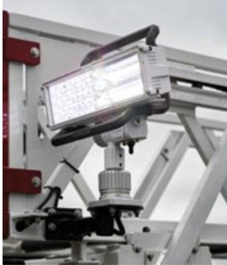
**TIP LIGHTING:** Multiple lighting choices are available at tip, 12 volts – 120 volts.
